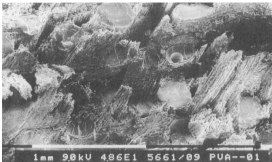
FIGURE 1(c). Fractured Surfaces Of Kapur-PMMA Composites
